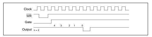
Figure 2-37. Mode 5 Timing Diagram
